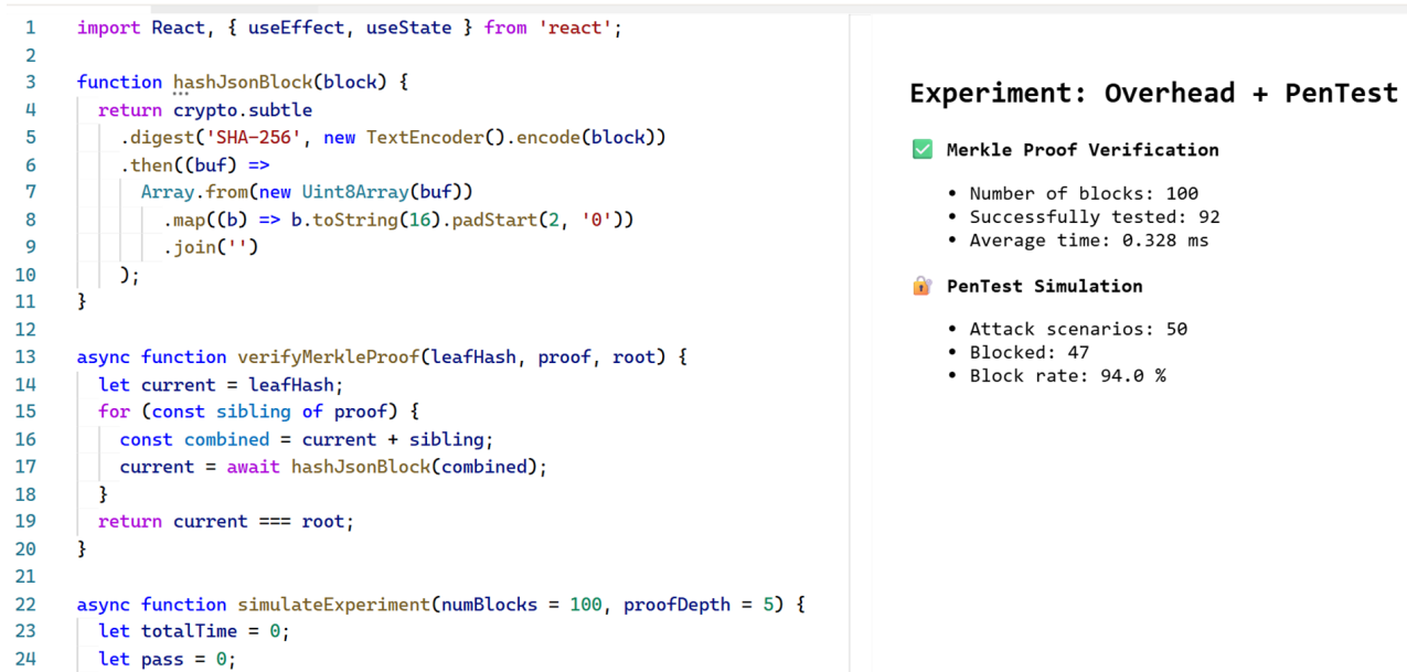
Figure 9. Fragment of React application for evaluating Merkle-proof verification overhead and results of PenTest scanning
