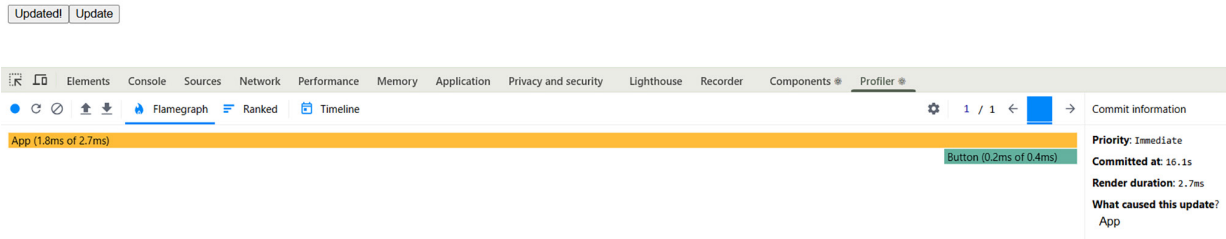
Figure 8. Profiling of rendering time of App and Button components in React DevTools
